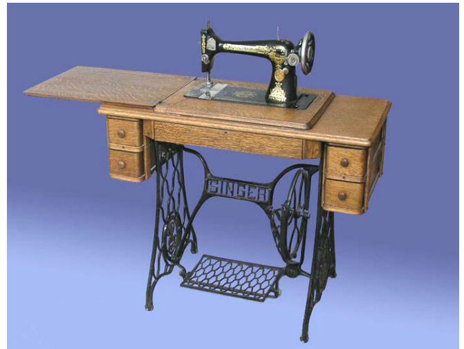
Treadle (foot-powered) sewing machine that Sarah used to sew 400 sets of burial clothes
